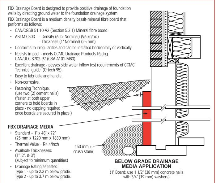
**Ontario Building Code:** FBX Drainage Board is designed and manufactured to meet the mineral fibre drainage layer requirements of the Ontario Building Code: ARTICLE 9.14.2.1 (2.1) (a).
